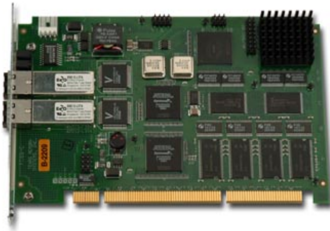
Figure A-2 FC-400 Dual Channel 4-Gigabit Fibre Channel Controller
