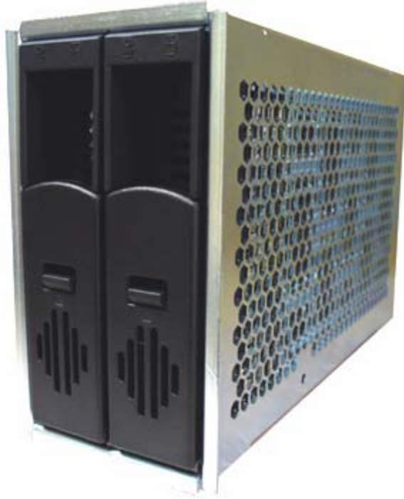
Figure A-5 Hard Drives in Sleds
