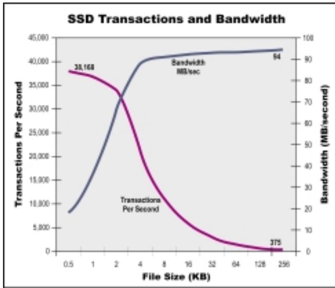
FIGURE 2: RAID TRANSACTIONS PER SECOND AND BANDWIDTH
